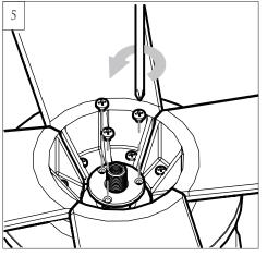
Remove the set screws from the plate on motor. Keep screws
