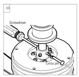
**Helpful hint:** For easy assembling of the cross pin **on the next installation step**. After slip downrod into the motor yoke, carefully insert a Phillips screwdriver through the yoke and downrod (**don't damage the lead wires**) as a guide and then push the cross pin and pull the screwdriver in the meantime as shown in the illustration.
