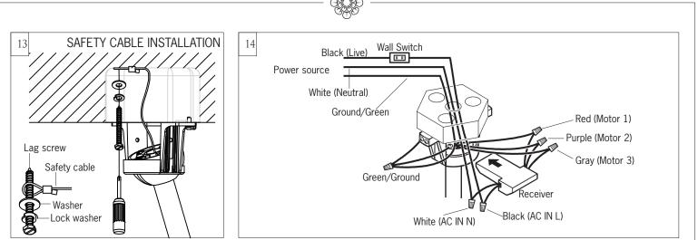
Safety cable must be installed into the house structure using 3" lag screws, washers, and lock washers provided, required for outdoor applications and in Canada (All fans installed in Canada), and for USA fan and light kit combinations over 35lbs.
