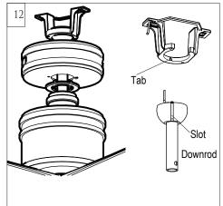
Install ball end of downrod into mounting bracket opening. Align (engage) slot on ball with tab on mounting bracket. **Warning:** Failure to align slot on ball with tab may result in serious injury. **Important**: If using the angle mount, make sure open end of mounting bracket is installed facing the higher point of the ceiling and make sure the ceiling angle is not steeper than 20°. Longer downrod may be necessary allowing the fan blades to rotate without obstructions.
