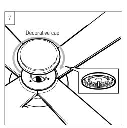
Install a decorative plate onto the adapter by turning clockwise till tight.
