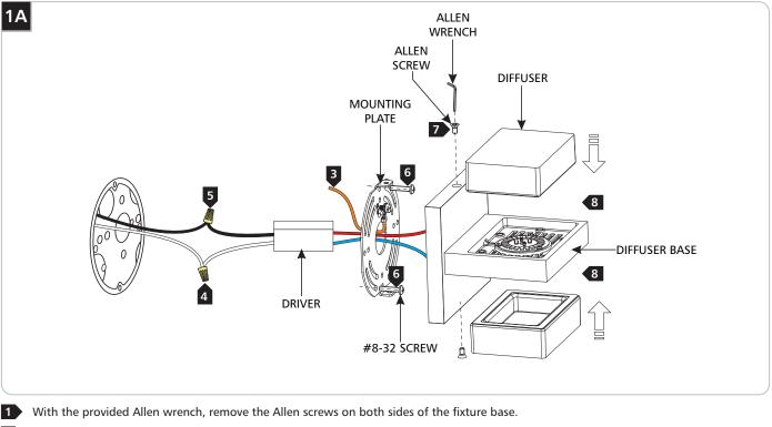
2 Remove the mounting plate from the back of the fixture.
