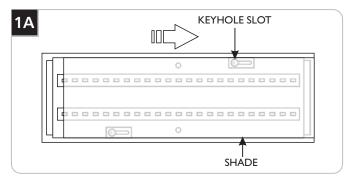
1 Remove the shade by sliding it all the way over to release it from the keyhole slot, then carefully pull it straight out.
