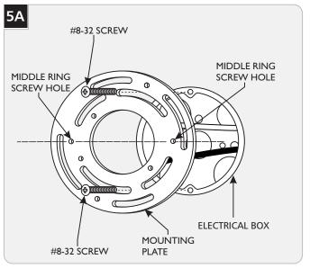
1 Align the two screw holes in the middle ring of the mounting plate horizontally and secure it to the electrical box with the two #8-32 screws provided.
