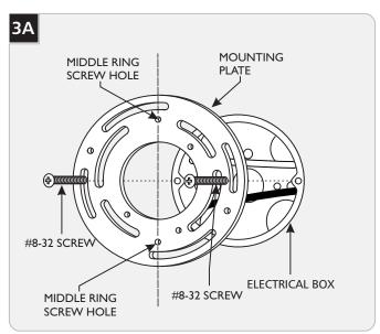
Align the two screw holes in the middle ring of the mounting plate vertically and secure it to the electrical box with the two #8-32 screws provided.
