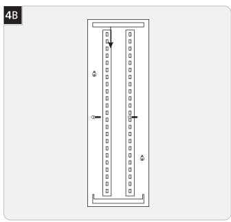
**NOTE:** Ensure that the shade will slide down to lock in place.
