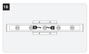
6 Secure the backplate to the electrical box with the two long #8-32 screws provided.
