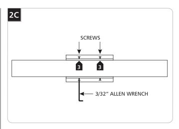
Tighten the four screws on both sides of the backplate with a 3/32" Allen wrench.
