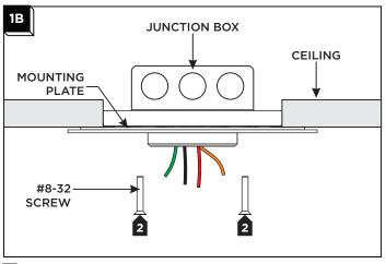
• Secure the mounting plate to the junction box with the #8-32 screws.
