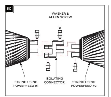
3 Use the isolating connector to connect two separately powered strings/fixtures using the washers and Allen screws. Tighten the Allen screws until snug.
