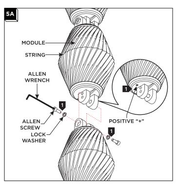
Connect strings together by using the washers and Allen screws making sure to match the polarity. Tighten the Allen screws until snug. **Only connect up** to 2' strings at a time (8 modules max).
