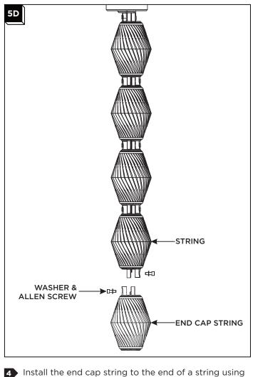
Install the end cap string to the end of a string using the washers and Allen screws making sure to match the polarity. Tighten the Allen screws until snug.
