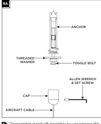
Disassemble stand-off assembly by unscrewing the cap from the threaded washer, then removing threaded washer and toggle bolt.
