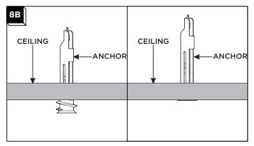
2 Install the anchor to the ceiling up to the threads. Screw it in the rest of the way.
