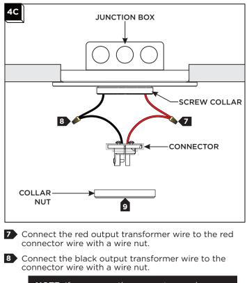
**NOTE:** If necessary, the connector can be rotated (180° maximum) to position its direction according to how the fixture will be hung/swagged.
