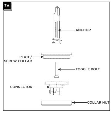
Disassemble stand-off assembly by unscrewing the collar nut and removing toggle bolt.
