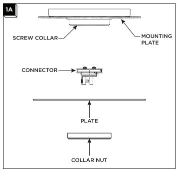
Remove the mounting plate from the canopy by unscrewing the collar nut from the screw collar.
