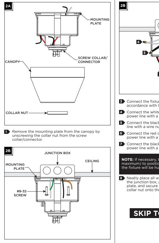
2 Secure the mounting plate to the junction box with the #8-32 screws.
