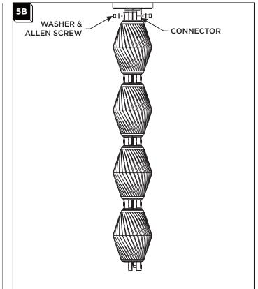
Install the increment to the connector using the washers and Allen screws making sure to match the polarity. Tighten the Allen screws until snug. Repeat as necessary. Do not attempt to hang the full length of string (more than 2' increments or 8 modules) at a time. Do not exceed a maximum of 20' of string per power feed point.
