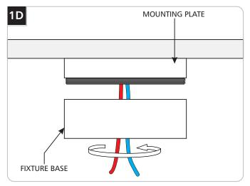
Feed the transformer wires through the fixture base and tightly reinstall it onto the mounting plate.
