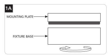
1 Unscrew the mounting plate from the fixture base.
