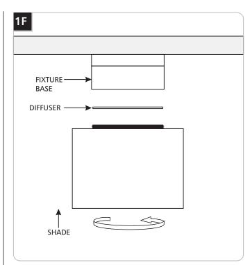
10 Place the diffuser into the fixture base and completely screw the shade into the base.
