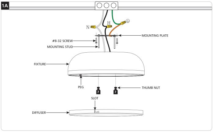
1 Remove the diffuser from the fixture by turning it clockwise, then pulling out of the fixture.
