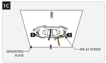
Secure the mounting plate to the junction box with 2 #8-32 screws.
