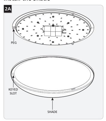
1 Align the pegs on the mounting plate with the keyed slots on the shade, push the shade onto the pegs, and rotate it to tightly secure in place.
