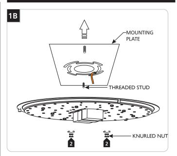
Remove the mounting plate from the fixture base by unscrewing the two knurled nuts from the two threaded studs.
