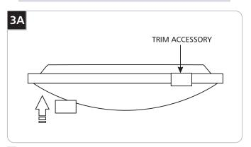
Attach the trim accessories to the rim of the shade. Imbedded magnets will allow the accessories to snap into place.
