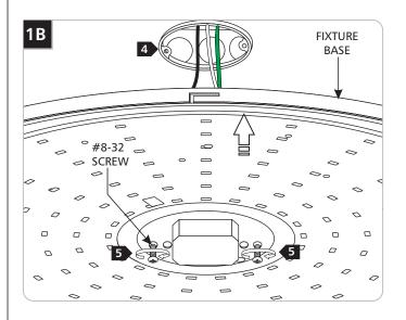
**Note**: depending on the dimensions of the J-box, you may use either the inner or outer through holes.
