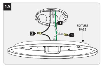
Ground the fixture in accordance with local electrical codes.
