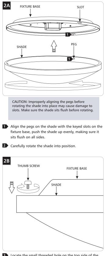
Locate the small threaded hole on the top side of the shade.
