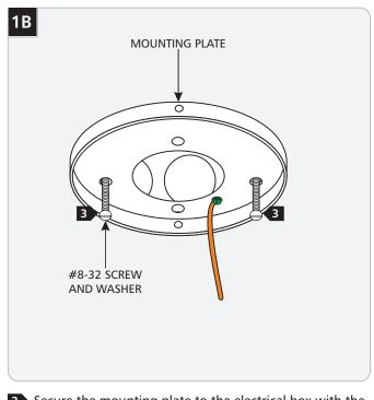
Secure the mounting plate to the electrical box with the #8-32 screws provided.
