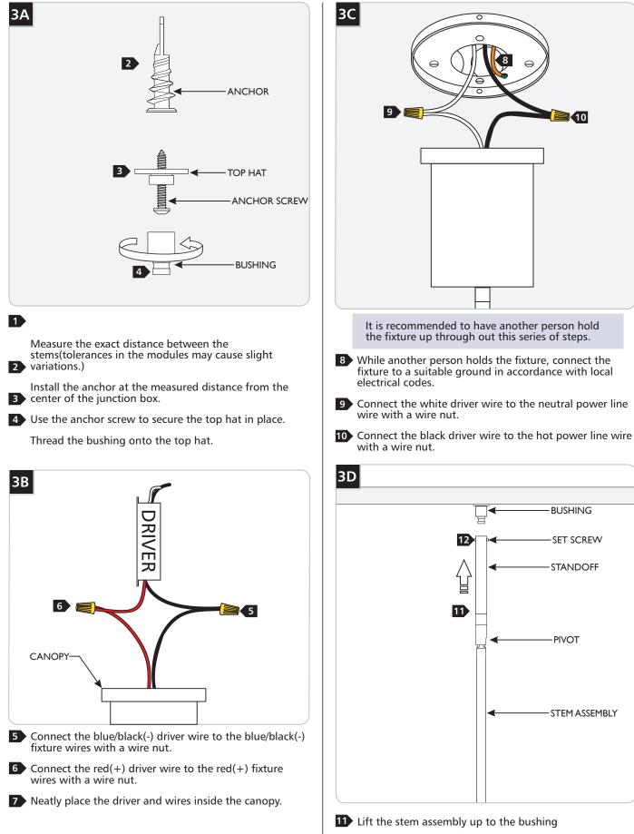
12 Screw the two set screw into place.
