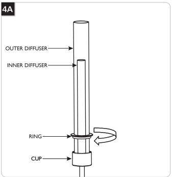
Insert the inner diffuser into the cup followed by the outer diffuser, then slide the ring over the outer diffuser and screw it into the cup to secure in place. Repeat for remaining diffusers.
