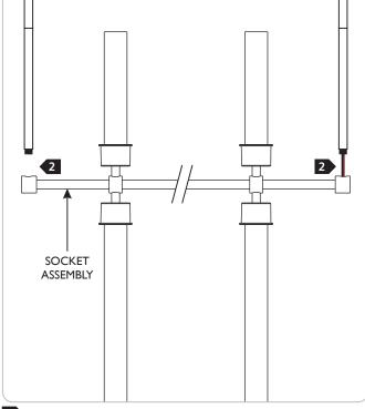
2 Feed the fixture wires through the stem assembly, then screw both stem assemblies onto the socket assembly.
