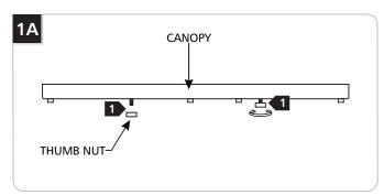
1 Separate the mounting plate from the canopy by first unscrewing and removing the two thumb nuts.
