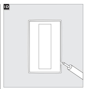
For wet locations, caulk around the base with waterproof construction sealant.
