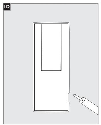
**For wet locations**, caulk around the base with waterproof construction sealant.
