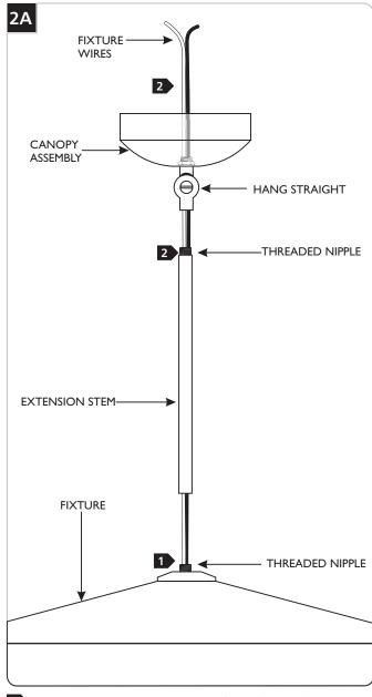
Determine the wanted length of the fixture, if necessary, feed the fixture wires through the stems and tighten stems completely to the threaded nipple on the fixture.
