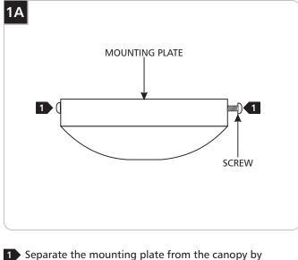
Separate the mounting plate from the canopy by removing the two screws.
