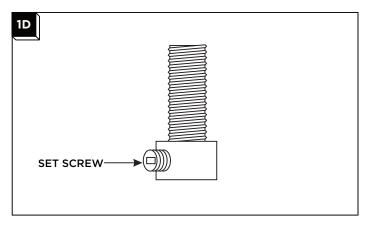
6 Loosen (Do Not Remove) the set screw on the strain relief.
