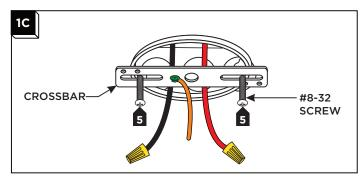
Mount the crossbar assembly to the junction box with the two provided #8-32 screws.
