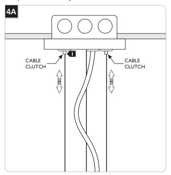
If necessary, adjust the aircraft cables until the fixture is level; feed the cable into the cable clutch to raise the fixture and push in on the cable clutch nipple to release the cable and lower the fixture.
