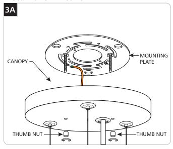
Remove the mounting plate from the assembly by unscrewing the two thumb nuts.
