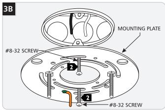
Secure the mounting plate to the electrical box with 2 #8-32 screws.
