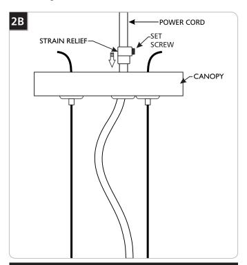
NOTE: The power cord does not support the fixture. For a casual "lazy cord" look, cut the power cord several inches longer that the drop height of the fixture.
