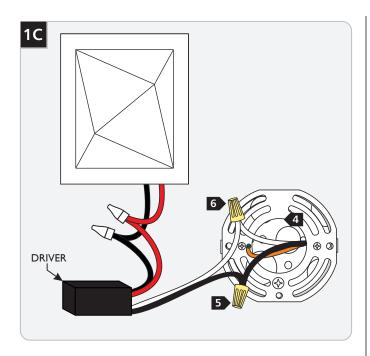
4 Connect the mounting plate ground wire to a suitable ground in accordance with local electrical codes.
