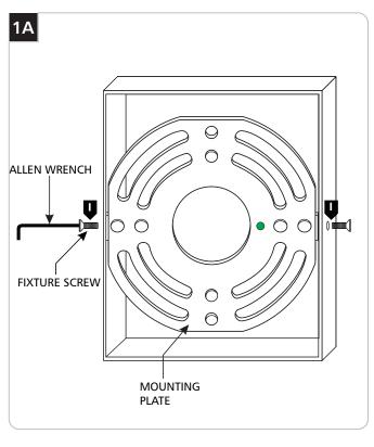
Remove the fixture screws located on both sides of the fixture base with the provided Allen wrench.
