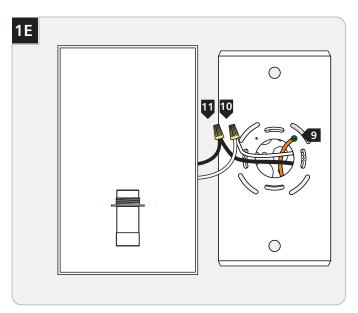
Onnect the mounting plate ground wire to a suitable ground according to local electrical codes.
