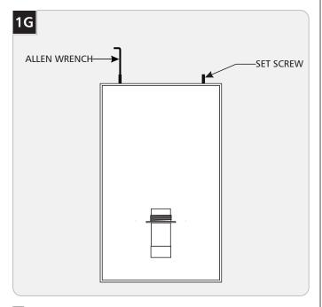
With the allen wrench, tighten the set screws to secure the fixture to the mounting plate.
