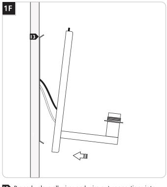
Properly place all wires and wire nut connections into the electrical box.
