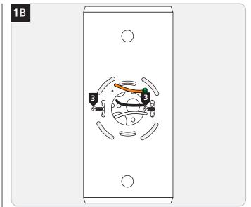
3 Level the mounting plate and secure it to the electrical box with the two #8-32 screws provided.
