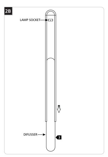
Slide out the diffuser completely to access the lamp sockets.
