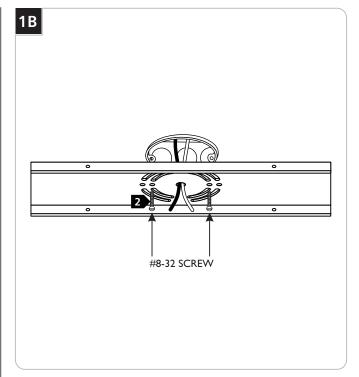
Attach the mounting plate to the electrical box using the two #8-32 screws provided.
