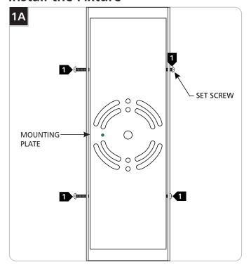
1 Unscrew the four set screws from the canopy and remove the mounting plate.
