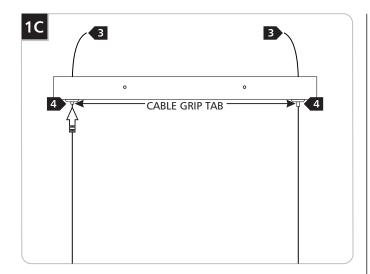
**NOTE:** When cutting the support cable to desired length, leave extra cable for fine tune leveling.
