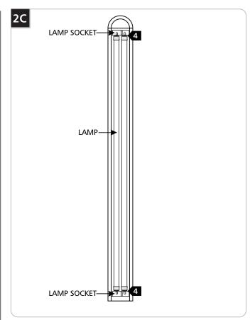
**CAUTION:** To reduce the risk of a burn or electric shock during relamping, disconnect the power to the fixture.
