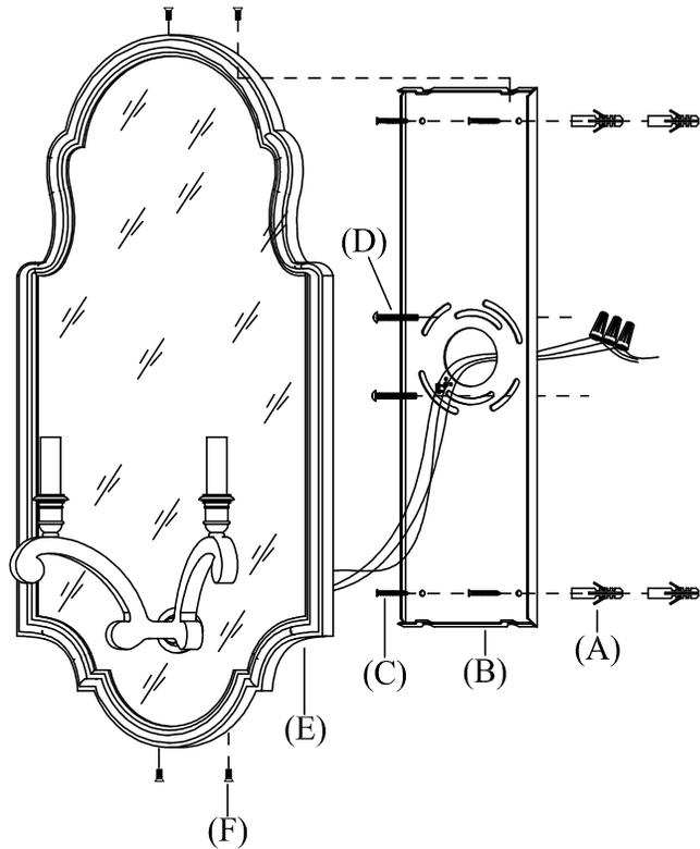
1. Remove mounting plate (B) from fixture base (E) by removing base screws (F).
