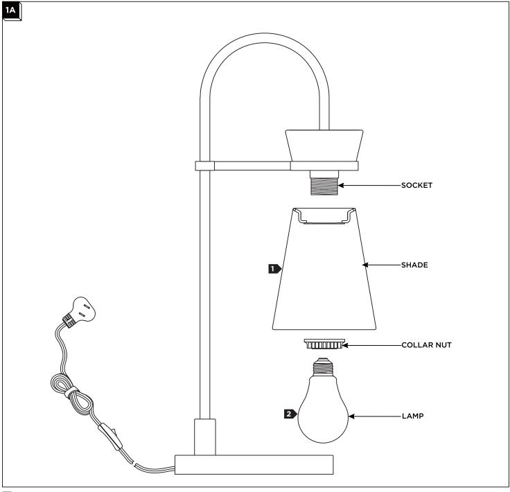
Place the shade over the socket and secure it in place by screwing the collar nut onto the socket.
