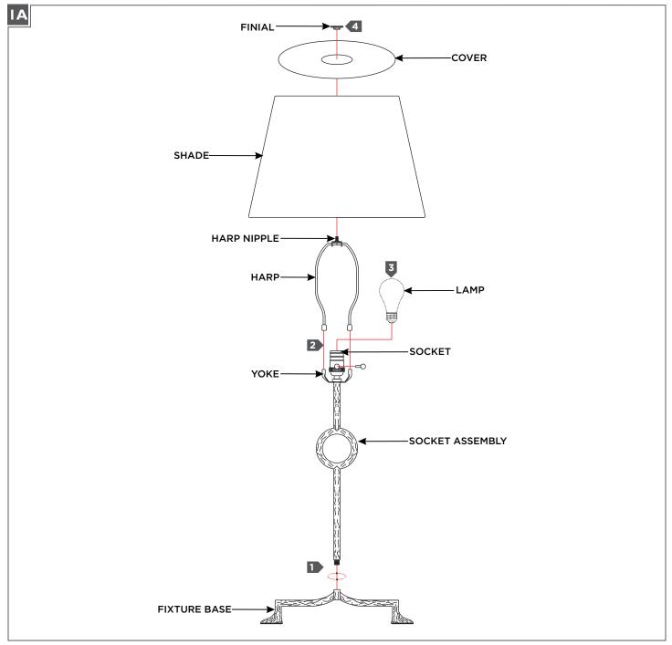
**1** Screw the socket assembly into the fixture base.
