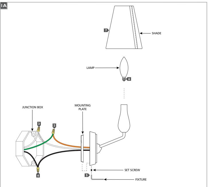
**I** Secure the mounting plate to the junction box.
