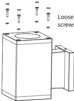
FIG.5 Loosen the fixture screws and gaskets
