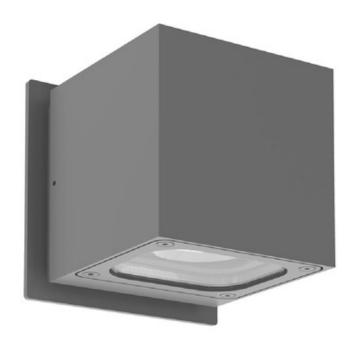
SHADE COLOR Clear **BODY FINISH** Graphite WATTAGE 15W DIMMER Not Dimmable DIMENSIONS 4"W x 4"H x 4.5"D INTEGRATED LED MODULE LAMP 1 x LED/120-277V LED Technical Information LUMINOUS FLUX 840 lumens LUMENS/WATT 56.00 LAMP COLOR 3000K COLOR RENDERING 80 CRI SPEC # KZC1034017
