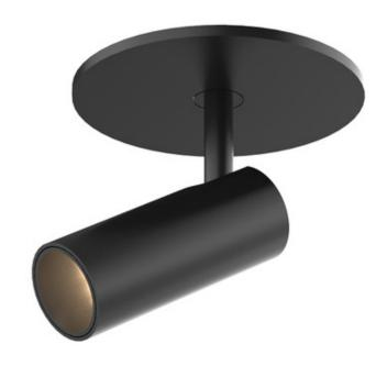
SHADE COLOR Clear **BODY FINISH** Black WATTAGE 4W DIMMER Low Voltage Electronic DIMENSIONS 2.38"W x 3.75"H INTEGRATED LED MODULE LAMP 1 x LED/120V LED Technical Information LUMINOUS FLUX 178 lumens LUMENS/WATT 44.50 LAMP COLOR 3000K COLOR RENDERING 90 CRI
