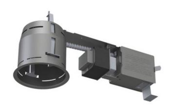
TRIM COLOR **BODY FINISH** Galvanized Steel WATTAGE 35W DIMMER Low Voltage Magnetic DIMENSIONS 13"L x 4.25"W x 4.5"H **BULB NOT INCLUDED** LAMP 1 x MR16/GU5.3 (bipin)/35W/12V Halogen MR16/GU5.3 (bipin)/12V LED Technical Information CEILING TYPE Drywall with Trim HOUSING TYPE Remodel NON IC HOUSING HEIGHT 5" APERTURE SIZE 3.500"
