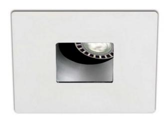
TRIM COLOR N/A **BODY FINISH** Matte White/ Anodized Reflector WATTAGE 50\\/ DIMMER Dimmable DIMENSIONS 4.25"W x 2.25"H x 4.25"D **BULB NOT INCLUDED** LAMP 1 x MR16/GU5.3 (bipin)/50W/12V Halogen 1 x MR16/GU5.3 (bipin)/12V LED 1 x MR16/GU10/9.8W/120V LED 1 x PAR16/Medium (E26)/8W/120V LED Technical Information FUNCTION Wall Washer CEILING TYPE Drywall with Trim APERTURE SHAPE Pinhole APERTURE SIZE 1700" SPEC # CLT106875
