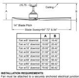
INSTALLATION REQUIREMENTS: Fan must be attached to a securely anchored electrical junction box capable of withstanding a load of at least 35 lbs.
