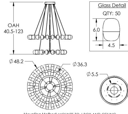
Mounting Method: MOUNTS TO J-BOX AND CEILING
