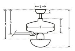
A 19.17 in (Low 17.1 in Angled 51.17 in) B 10.87 in (Low 8.87 in Angled 42.87 in) C 2.75 in D 12.07 in E 6.49 in F 19.17 in (Low 17.17 in Angled 51.17 in) G 4.59 in
