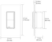
$\label{eq:Note: Note: Requires a U.S. wallbox 2 \% in (57 mm) deep minimum.}$   $\label{eq:Note: The accessory switch ST-AS does not have the light bar pictured.}$
