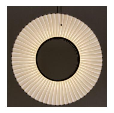
SHADE COLOR Ivory Ribbon BODY FINISH Black WATTAGE 28W DIMMER 0-10V DIMENSIONS 19.6"W x 19.6"H INTEGRATED LED MODULE LAMP 1 x LED/28W/120V LED Technical Information LUMINOUS FLUX 2800 lumens LUMENS/WATT 100.00 LAMP COLOR 2700K COLOR RENDERING 85 CRI
