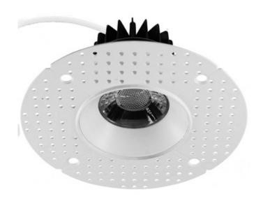
TRIM COLOR N/A **BODY FINISH** Matte White WATTAGE 12W DIMMER Low Voltage Electronic DIMENSIONS 3.5"W x 3.25"H INTEGRATED LED MODULE 1 x LED/12W/120V LED LAMP Technical Information LUMINOUS FLUX 800 lumens LUMENS/WATT 66.67 LAMP COLOR CCT Select COLOR RENDERING 90 CRI BEAM ANGLE 38° FUNCTION Downlight CEILING TYPE Drywall Trimless/Flush HOUSING TYPE Remodel IC Airtight HOUSING HEIGHT 3" SPEC # BEA1161711
