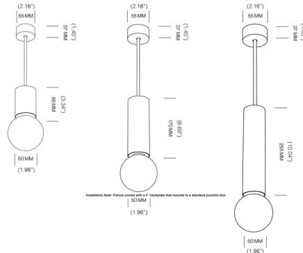
Installation Note: Fixture comes with a 4" backplate that mounts to a standard junction box.
