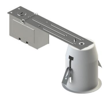
TRIM COLOR N/A BODY FINISH Aluminum WATTAGE 50W DIMMER Standard 120V DIMENSIONS 12.63"L x 3.5"W x 4.13"H **BULB NOT INCLUDED** LAMP 1 x MR16/GU10/50W/120V Halogen 1 x MR16/GU10/120V LED Technical Information CEILING TYPE Drywall with Trim HOUSING TYPE Remodel NON IC HOUSING HEIGHT APERTURE SIZE 3.000"
