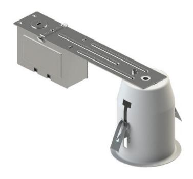
TRIM COLOR N/A BODY FINISH Aluminum WATTAGE 50W DIMMER Dimmable DIMENSIONS 12.75"L x 4"W x 4.63"H **BULB NOT INCLUDED** LAMP 1 x MR16/GU10/50W/120V Halogen 1 x MR16/GU10/120V LED Technical Information CEILING TYPE Drywall with Trim HOUSING TYPE Remodel NON IC HOUSING HEIGHT 5" APERTURE SHAPE Round SPEC # EUF184740
