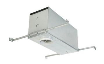
TRIM COLOR N/A **BODY FINISH** Aluminum WATTAGE 7\// DIMMER Standard 120V DIMENSIONS 15.5"L x 6"W x 7.25"H **BULB NOT INCLUDED** LAMP 1 x MR16/GU10/7W/120V LED Technical Information CEILING TYPE Drywall with Trim HOUSING TYPE New construction IC HOUSING HEIGHT 8" APERTURE SIZE 4.000" SPEC # EUF184747
