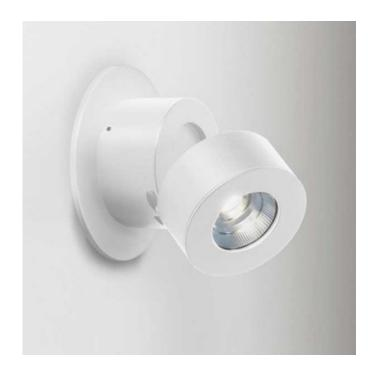
SHADE COLOR N/A **BODY FINISH** White WATTAGE 6.2W DIMMER Dimmable DIMENSIONS 3.1"W x 3.5"H INTEGRATED LED MODULE LAMP 1 x LED/6.2W/120V LED Technical Information LAMP COLOR 2700K COLOR RENDERING 80 CRI BEAM ANGLE 22°
