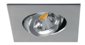
TRIM COLOR Clear BODY FINISH **Brushed Nickel** WATTAGE 16\\\ DIMMER Dimmable DIMENSIONS 4.9"W x 3.75"H x 4.9"D INTEGRATED LED MODULE LAMP 1 x LED/120V LED 1 x LED/120V LED Technical Information LUMINOUS FLUX 1575 lumens LUMENS/WATT 98.44 LAMP COLOR 3000K COLOR RENDERING 90 CRI BEAM ANGLE 47° LAMP LIFE 50000 hours **FUNCTION** Adjustable Accent CEILING TYPE Drywall with Trim APERTURE SHAPE Square SPEC # CLT233516
