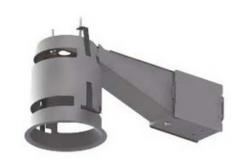
TRIM COLOR N/A **BODY FINISH** Galvanized Steel WATTAGE 16\\\ DIMMER 0-10V DIMENSIONS 13.5"W x 5.5"H x 5.2"D INTEGRATED LED MODULE LAMP 1 x LED/120V LED Technical Information LUMINOUS FLUX 1500 lumens LUMENS/WATT 93.75 CEILING TYPE Drywall with Trim HOUSING TYPE Remodel NON IC SPEC # CLT234228
