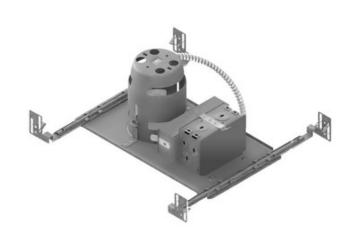
TRIM COLOR N/A **BODY FINISH** Galvanized Steel WATTAGE 23/// DIMMER Low Voltage Electronic DIMENSIONS 13.5"W x 5.5"H x 7.4"D INTEGRATED LED MODULE LAMP 1 x LED/120V LED Technical Information LUMINOUS FLUX 2000 lumens LUMENS/WATT 86.96 CEILING TYPE Drywall with Trim HOUSING TYPE New Construction NON IC
