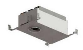
TRIM COLOR N/A **BODY FINISH** Galvanized Steel WATTAGE 23W DIMMER 0-10V DIMENSIONS 19.5"W x 7.1"H x 10"D INTEGRATED LED MODULE LAMP 1 x LED/23W/120V LED Technical Information LUMINOUS FLUX 2000 lumens LUMENS/WATT 86.96 CELLING TYPE Drywall with Trim HOUSING TYPE New construction IC
