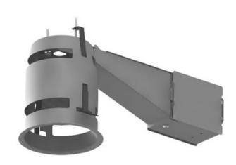
TRIM COLOR N/A BODY FINISH Galvanized Steel WATTAGE 23/// DIMMER Low Voltage Electronic DIMENSIONS 13"W x 5.5"H x 4.63"D INTEGRATED LED MODULE LAMP 1 x LED/120V LED Technical Information LUMINOUS FLUX 2000 lumens LUMENS/WATT 86.96 CEILING TYPE Drywall with Trim HOUSING TYPE Remodel NON IC SPEC # CLT235488
