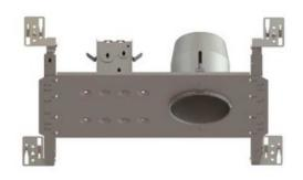
TRIM COLOR N/A BODY FINISH N/A WATTAGE 10W DIMMER Low Voltage Electronic DIMENSIONS 13.5"L x 7.3"W x 4.5"H **BULB NOT INCLUDED** LAMP 1 x MR16/GU10/10W/120V LED Technical Information FUNCTION Downlight CEILING TYPE Drywall with Trim HOUSING TYPE New construction IC Airtight HOUSING HEIGHT
