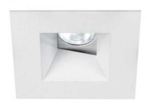
SHADE COLOR N/A **BODY FINISH** White WATTAGE 21 5\\\/ DIMMER Dimmable DIMENSIONS 5.25"W x 5.25"D INTEGRATED LED MODULE LAMP 1 x LED/21.5W/120V LED Technical Information LUMINOUS FLUX 950 lumens LUMENS/WATT 44.19 LAMP COLOR 2700K COLOR RENDERING 90 CRI BEAM ANGLE 30° FUNCTION Adjustable Accent CEILING TYPE Drywall with Trim APERTURE SHAPE Square SPEC # WAC362176
