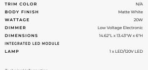
Technical Information LUMINOUS FLUX 1189 lumens LUMENS/WATT 59.45 LAMP COLOR 2700K COLOR RENDERING 90 CRI BEAM ANGLE 32° LAMP LIFE 50000 hours FUNCTION Adjustable Accent HOUSING TYPE New construction IC HOUSING HEIGHT SPEC # CLT371720
