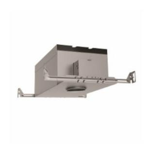
TRIM COLOR N/A **BODY FINISH** Galvanized Steel WATTAGE 50W DIMMER Low Voltage Magnetic DIMENSIONS 19.5"L x 10"W x 7.1"H **BULB NOT INCLUDED** LAMP 1 x MR16/GU5.3 (bipin)/50W/12V Halogen MR16/GU5.3 (bipin)/12V LED Technical Information CEILING TYPE Drywall with Trim HOUSING TYPE New construction IC Airtight HOUSING HEIGHT APERTURE SIZE 4.000"
