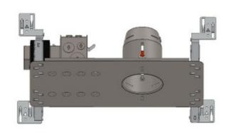
TRIM COLOR N/A BODY FINISH Galvanized Steel WATTAGE 35\// DIMMER Low Voltage Magnetic DIMENSIONS 11.4"L x 7.3"W x 4.6"H **BULB NOT INCLUDED** LAMP MR16/GU5.3 (bipin)/35W/12V Halogen MR16/GU5.3 (bipin)/12V LED Technical Information CEILING TYPE Drywall with Trim HOUSING TYPE New Construction NON IC HOUSING HEIGHT APERTURE SIZE 3.000"
