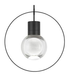
**BODY FINISH** Black WATTAGE 14 5W DIMMER Low Voltage Electronic DIMENSIONS 79.6"L x 12.8"W x 13.3"H INTEGRATED LED MODULE LAMP 1 x LED/120V LED Technical Information LUMINOUS FLUX 290 lumens LUMENS/WATT 20.00
